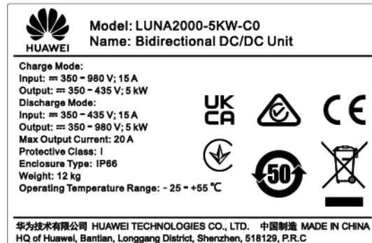
Nameplate of a battery expansion module
