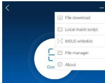
**Step 2** Download the device upgrade package and grid code when an update is detected.
