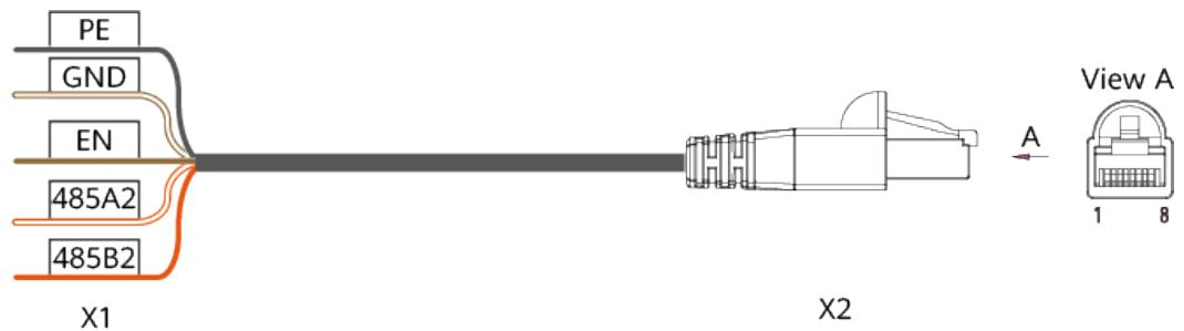
**Table 6-3** Signal cable connection (purchased from the supplier, type 2) between the battery and the inverter
