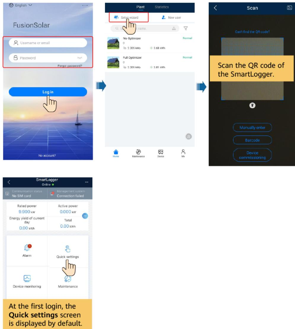
**Step 2** Tap **Quick settings** to set parameters for commissioning as prompted. For details about setting the battery working mode, see [3 "Application Scenarios and Settings"](#).
