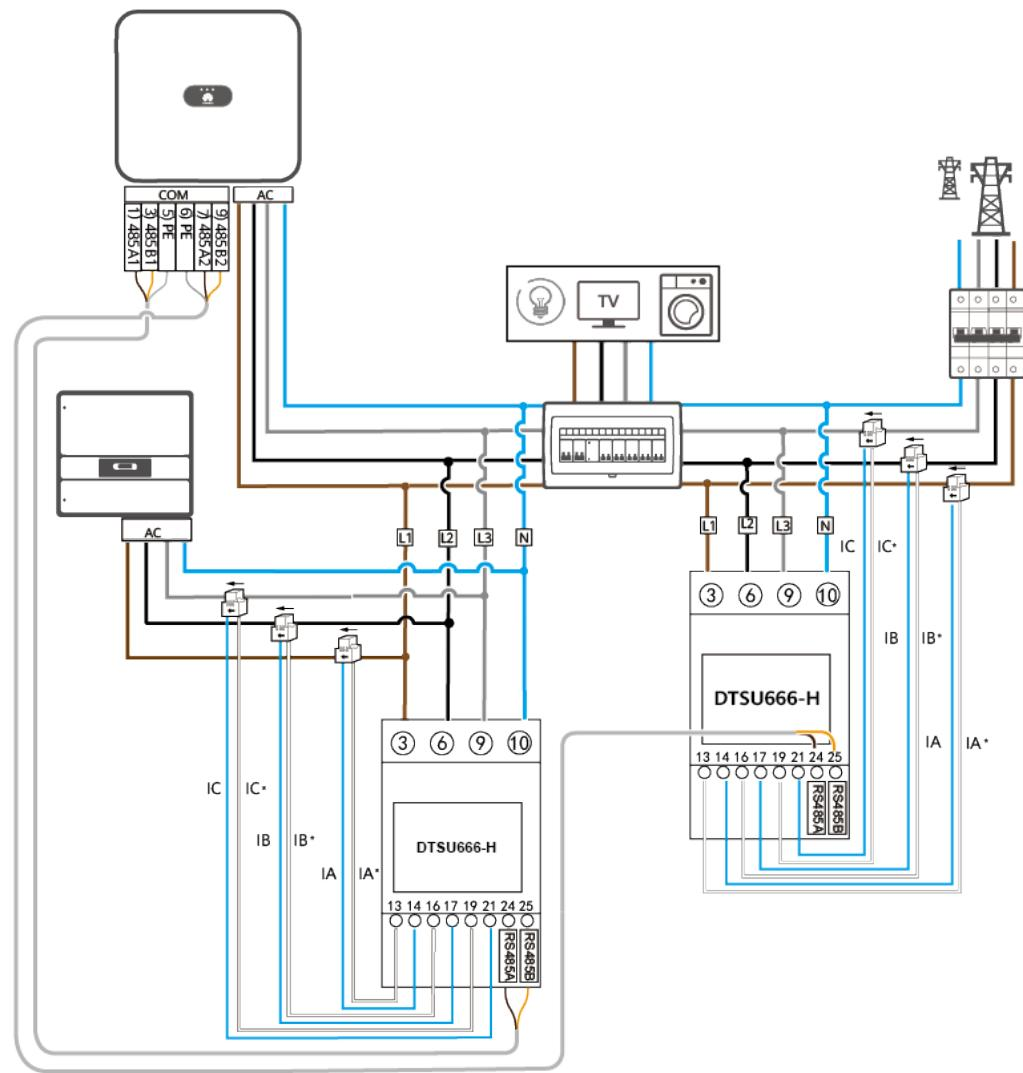
**Table 4-16** Power meter cable connections for SUN2000-(3KTL-10KTL)-M1
