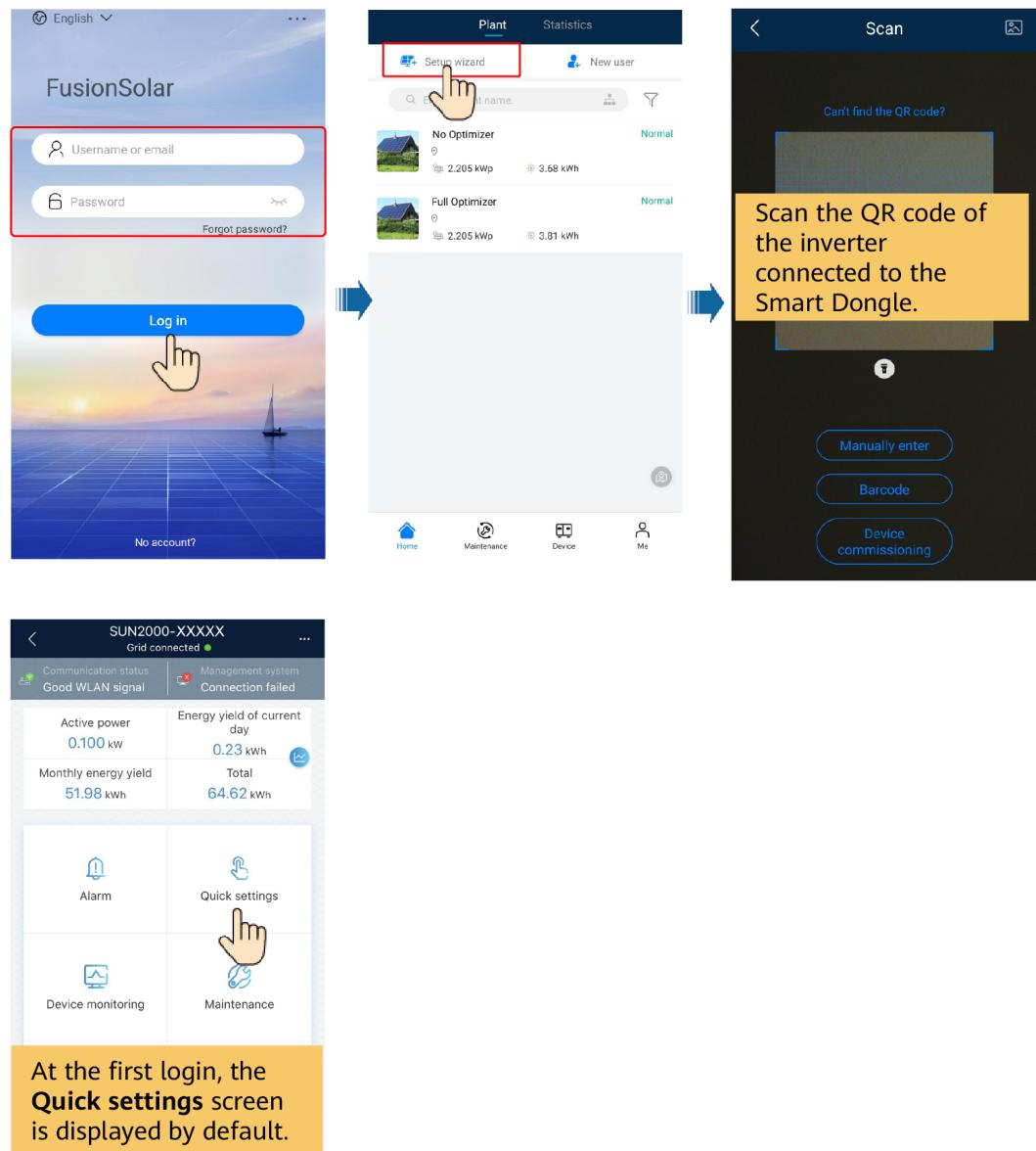
**Step 2** Tap **Quick settings** to set parameters for commissioning as prompted. For details about setting the battery working mode, see [Application Scenarios and Settings](#).
