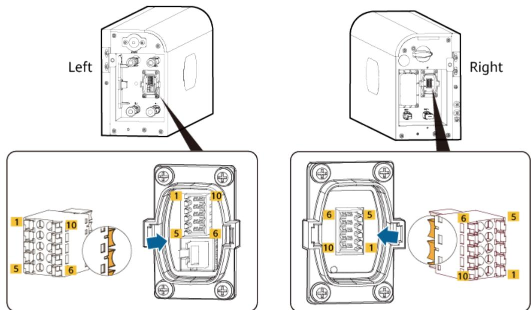
**Figure C-2** Inverter connected to two batteries (method 1)
