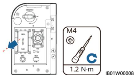
**Step 3** Lift the fuse box opening, remove the fuse, insert a new fuse into the slot, and close the fuse box. If you hear a click sound and the bulge on the side is inside the box, the fuse box is properly installed.
