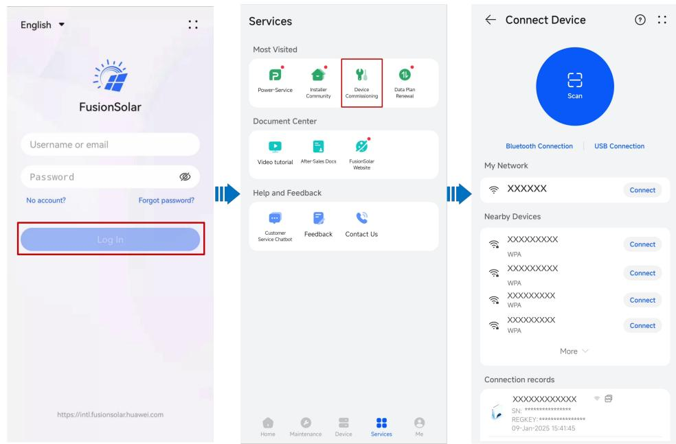
**Figure A-2** Method 2: mobile phone not connected to the Internet
