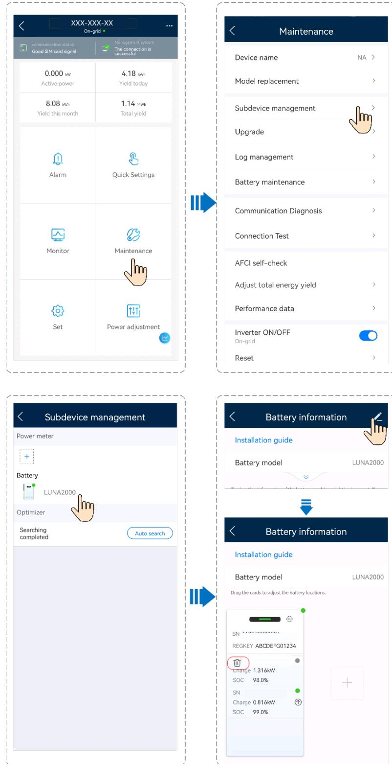
When the EMMA is used for networking, [connect to the EMMA on the app](#), tap **Monitor** on the home screen, select the connected inverter, choose **Maintenance** > **Subdevice management**, tap the ESS icon, and delete the offline power control module or battery expansion module.
