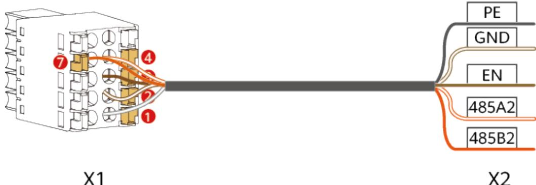
**Table 6-2** Signal cable connection (purchased from the supplier, type 1) between the battery and the inverter
