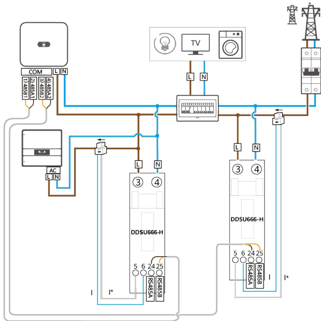
**Table 4-15** Power meter cable connections for SUN2000-(2KTL-6KTL)-L1
